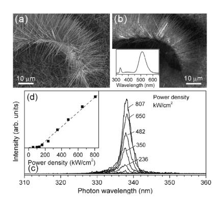
(a) SEM and (b) CL images of ZnS nanowire arrays on CdS nanoribbons. The inset is the corresponding CL spectrum. (c) PL spectra and (d) PL intensity of epitaxially grown nanostructures excited by different excitation power densities.
